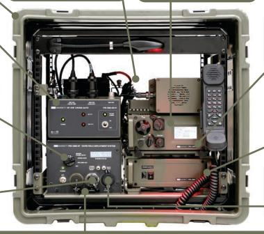
HF Modem for email fax and data over HF radio operation
