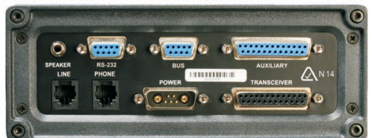
Barrett 2060 HF Telephone interconnect rear panel
